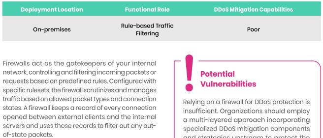
This qualifies the firewall as a stateful device, and like many other stateful devices, the firewall is vulnerable to saturation DDoS attacks such as HTTP attacks and SYN floods. While the firewall can sift through packets related to a DDoS attack, it's generally not optimized to handle the sheer volume of incoming packets that accompany such attacks. This results in the firewall quickly becoming overwhelmed, leading it to "fail closed" state, which leads to downtime.
